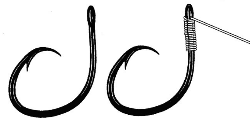
Figure 2: Unmodified circle hook (left) and circle hooks with wire appendage (right). Diagram by J. Javech, NOAA Fisheries
