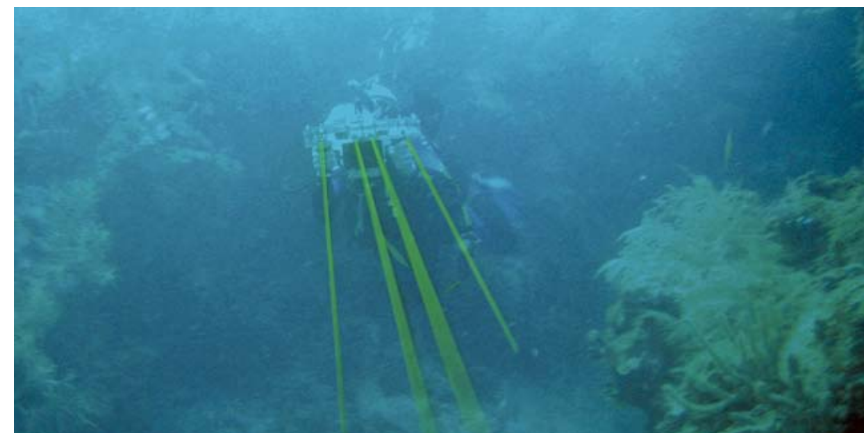
Figure 1: A laser sizing and ranging camera system developed for the reef fish visual census is employed in the Florida Keys.
