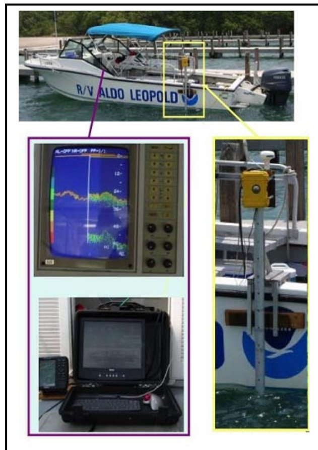
Figure 1: Survey vessel and QTCV equipment. Top panel shows the 25-foot research vessel used for data acquisition. Bottom left panel (in purple box) shows the echosounder and data capture screen. Bottom right panel (in yellow box) shows the gunwale-mounted pole used to support the acoustic transducer. Note the system is portable and easily installed, either temporarily, as shown here, or permanently, on virtually any vessel.
