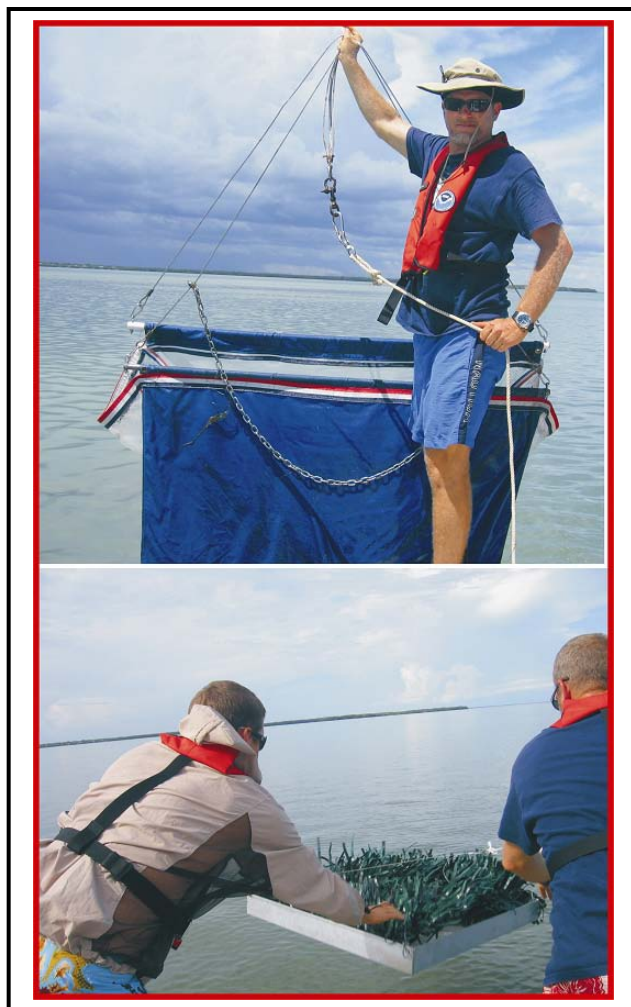
Figure 1: Sampling methods used in northern Florida Bay to collect early settlement stages of pink shrimp: Renfro trawl and settlement traps with artificial sea-grass.
