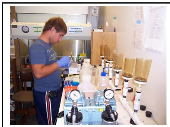
Figure 4: CIMAS graduate student filters beach water samples for molecular analysis of fecal indicator bacteria and pathogens as part of ground-truthing for the EPA-STREAMS Virtual Beach Project.
