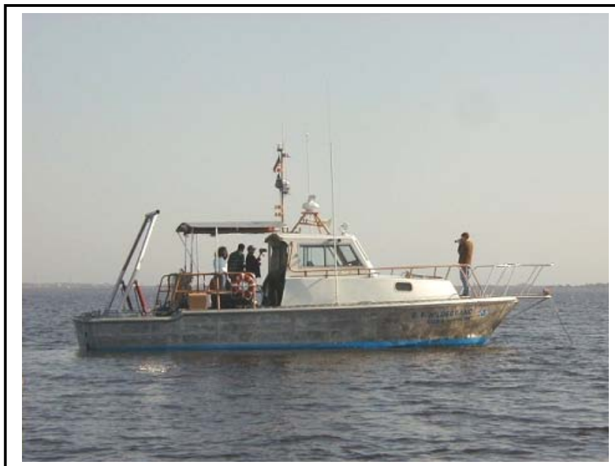
Figure 2. Side view of the NOAA R/V Hildebrand, a 41-foot Coast Guard utility boat formerly at the NOAA Beaufort laboratory. The boat will be used for the upcoming FACE water quality monitoring project in the waters off of SE Florida
