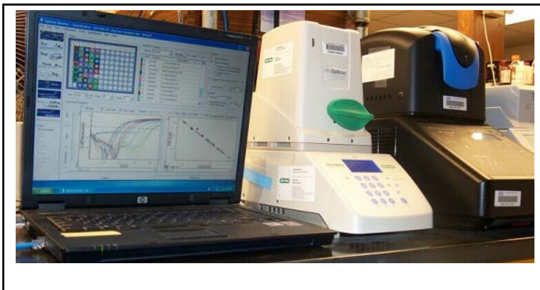
Figure 3: Image of real-time quantitative PCR instrumentation running a molecular assay to measure the amount of canine-source Bacteroides fecal indicator bacteria in beach water
