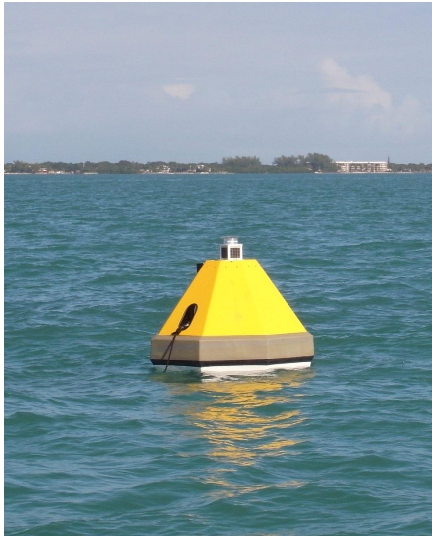
Figure 3: Top-side view of MAPCO2 buoy at Cheeca Rocks in the Florida Keys which is the site of the Atlantic Ocean Acidification Test bed.
