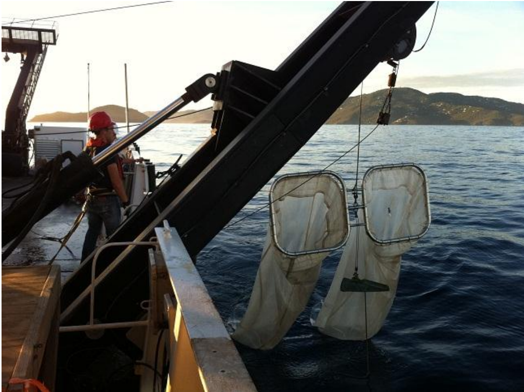
Figure 1: NOAA Core officer Aaron Maggied deploys bongo net aboard the NOAA ship Nancy Foster in the US Virgin Islands.
