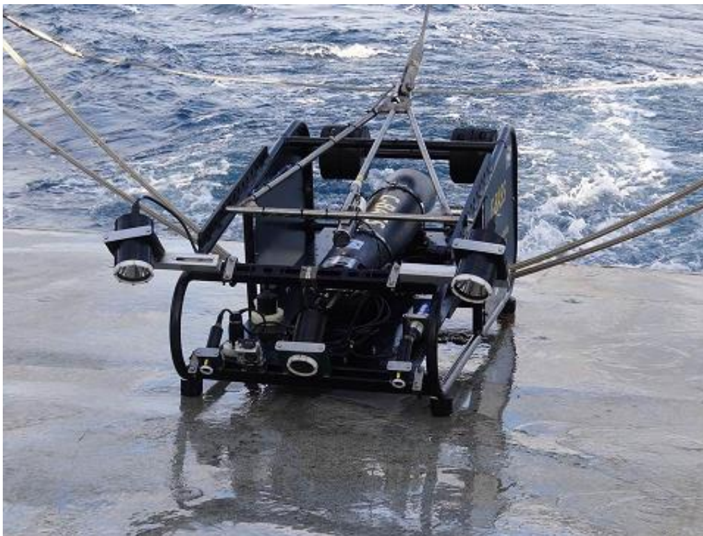
Figure 1: The C-BASS (Camera-Based Survey Sampling System) tow vehicle, prototype 1. In the front there are four cameras (1 digital and 3 analog) and two light strobes.
