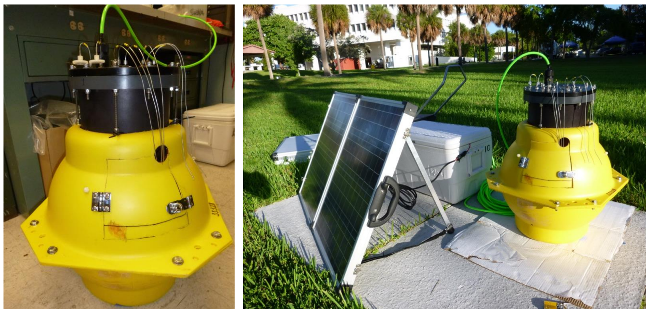
Figure 1. Submersible, solar-powered system for in-situ ammonium measurement in natural waters.
