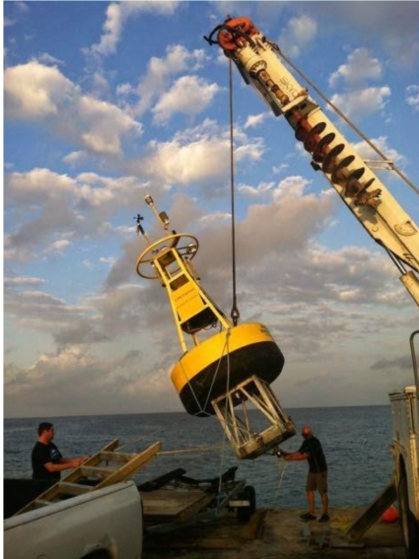
Figure 2: The CREWS buoy was brought to shore early in 2015 to troubleshoot a power failure.
